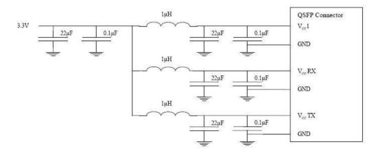
Figure 1. Host Board Power Supply Filtering
